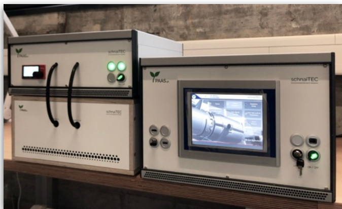
The PAAS-4 \lambda consists of separate optics, electronics and flow units that are prepared for 19" rack integration or desktop installation.
